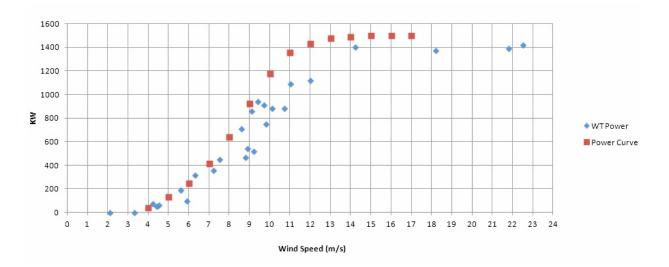
This graph shows blue diamonds highlighting values from the Hoosac noise testing report (plotted from the table on the left below) to represent the power output during testing. The red boxes come from the published power curve of the GE 1.5 sle wind turbine. The expected power output related to wind speed is shown in the table on the right below.
